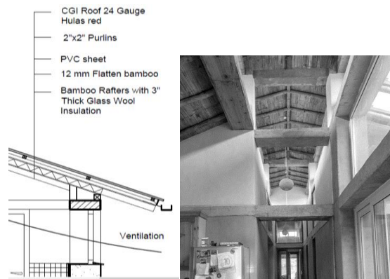
Figure 6: Roof details of Mato Ghar
