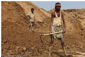
Photograph 1 Excavate the mud from which bricks are made (Mostafa, n.d.)
