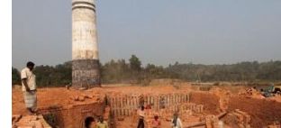
Photograph 4 Human labour involved in staking of green bricks and unloading of burnt brick.(Mostafa, n.d.)
